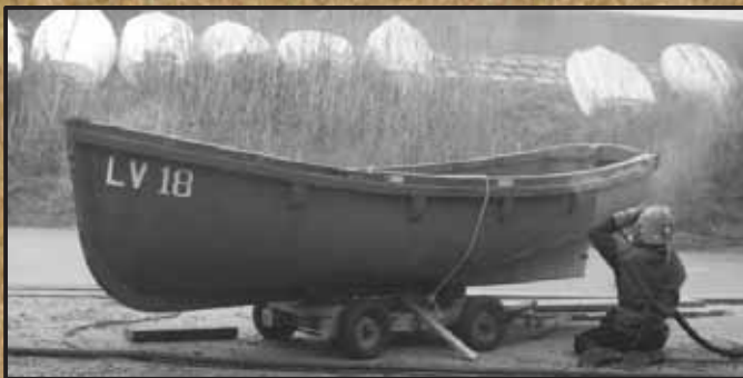
ORIGINAL LV18 BEING SAND BLASTED
